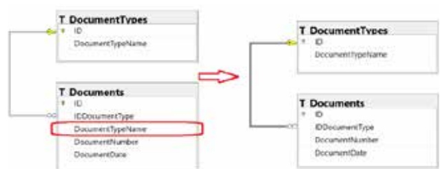
Fig. 4. Database diagram with/without redundant attribute
